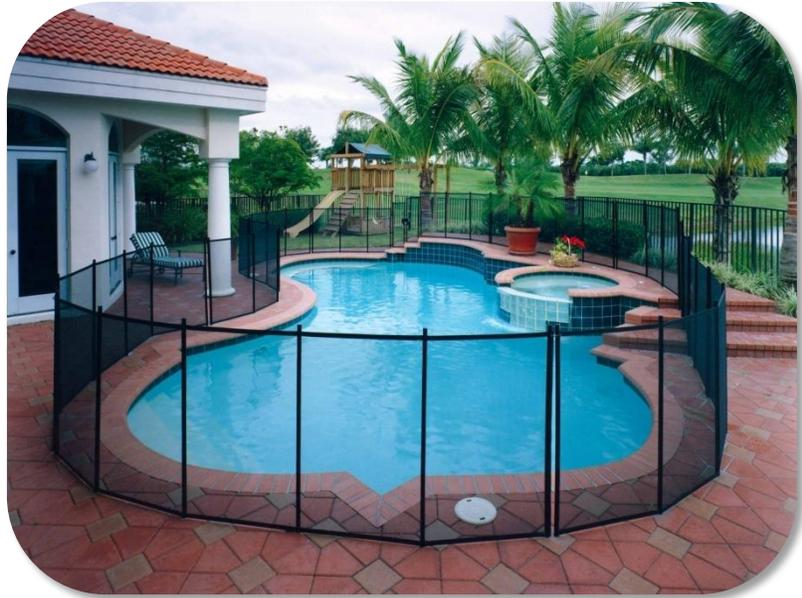
Pool fence is constructed of see through, polyester mesh mounted on aluminum or fiberglass support poles. The fence is placed into aluminum or plastic sleeves installed into your deck surface. The bottom border of the fence material should be flush to your deck so as to prevent a child from pushing under. The basic principle that keeps pool fence in place is bilateral tension and the fence should be checked periodically to insure that you have benefit of its full function.
